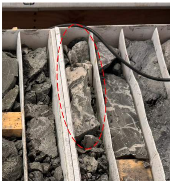
Figure 12-7: Variable mineralisation orientation for check sample ACDDH058 173.5–174 m prior to quarter-core sampling.
