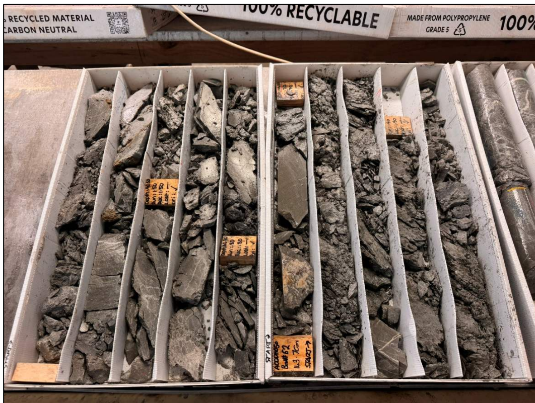
Figure 12-1: Example of core tray samples selected by the QP (Abraham Whaanga) for verification sampling (ACDDH050: Box 61 and Box 62).
