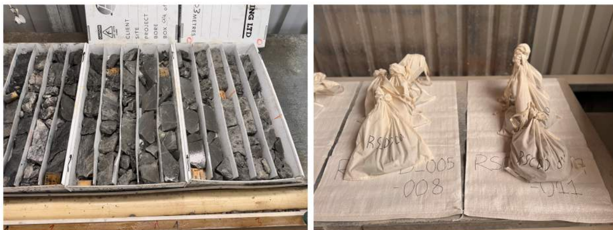
Figure 12-6: Quarter-core verification sampling conducted by RSC in January 2026: half-core verification samples prior to cutting (left); quarter-core check samples relabelled (right).
