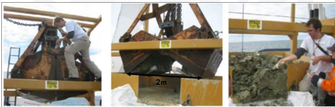
Figure 11-1: RV Dorado Discovery clamshell grab sample processing.
