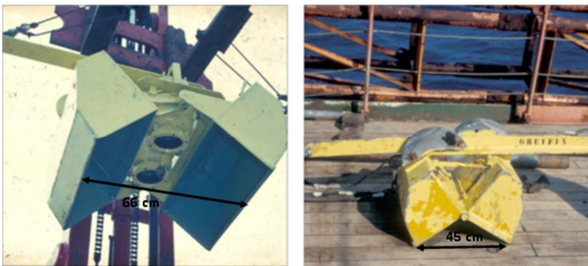
Figure 6-4: Large (left) and small (right) Van Veen grab samplers used to collect sediment samples aboard the RV Valdivia .
