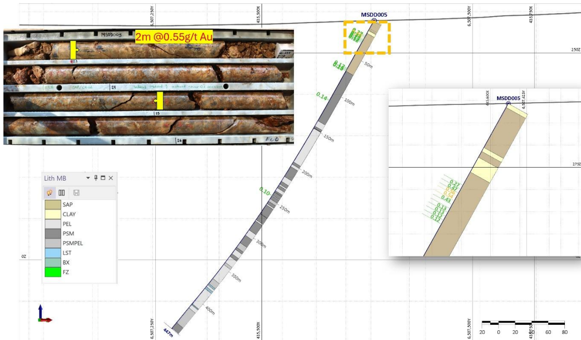
Figure A1.5: MSDD005 cross section looking North, showing Photon Assay results for Au>0.1g/t, including 2m @0.55g/t, from 23m to 25m.
