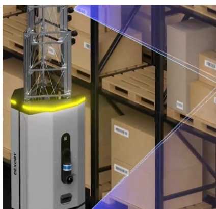
Dex can scan UPCs or licence plates to confirm the correct SKU is in the correct location
